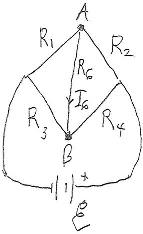
Remove the edge AB and find the equivalent emf  $\mathcal{E}_0$  in series with the internal resistance  $R_0$
