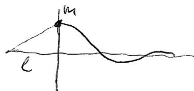
Next I want to look at a string with s.h.o. attached. In this situation the equations of motion are  $\ddot{u} = \partial_x^2 u$  for  $x \geq 0$  and  $m\ddot{u}_0 = -\frac{1}{l}u_0 + (\partial_x u)_0$ . Using the first, the second may be written  $(m\partial_x^2 u + \frac{1}{l}u - \partial_x u)_0 = 0$ , i.e. a sort of boundary condition with derivatives. Also there are limiting cases of interest:  $m=0$ ,  $l=\infty$ .
