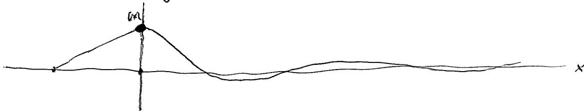
For  $x > 0$  we have a string of uniform density  $\rho$  and tension  $T$ ; let  $u(x, t)$  be the displacement. At  $x=0$  the string is attached to a mass  $m$  which in turn is joined by a <sup>thread</sup> (weightless string) to a point on the negative axis. Ignoring  $x > 0$  the mass is a simple harmonic oscillator whose motion is given by  $m(\ddot{y} + \omega_0^2 y) = 0$ , ~~where~~ where  $y = u(0, t)$ . The force on the mass due to the string is
