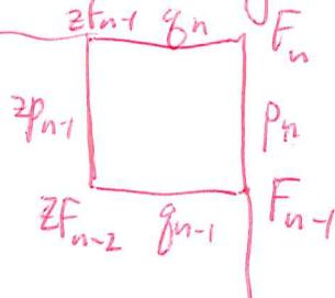
$$\begin{pmatrix} p_n \\ q_n \end{pmatrix} = \underbrace{\begin{pmatrix} a & b \\ c & d \end{pmatrix}}_{u(1,1)} \begin{pmatrix} zp_{n-1} \\ q_{n-1} \end{pmatrix}$$
