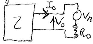
line as the resistance  $R_0 = \sqrt{\frac{L}{C}}$  with a noise generator  $V_n$ .
