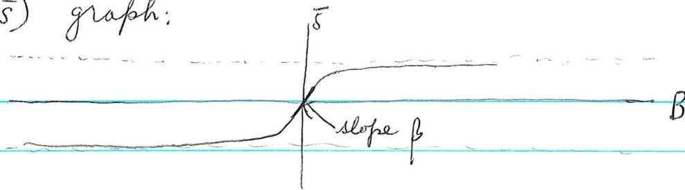
$$\bar{s} = \tanh \beta B \quad \text{or} \quad B = \frac{1}{\beta} \frac{1}{2} \log\left(\frac{1+\bar{s}}{1-\bar{s}}\right)$$
