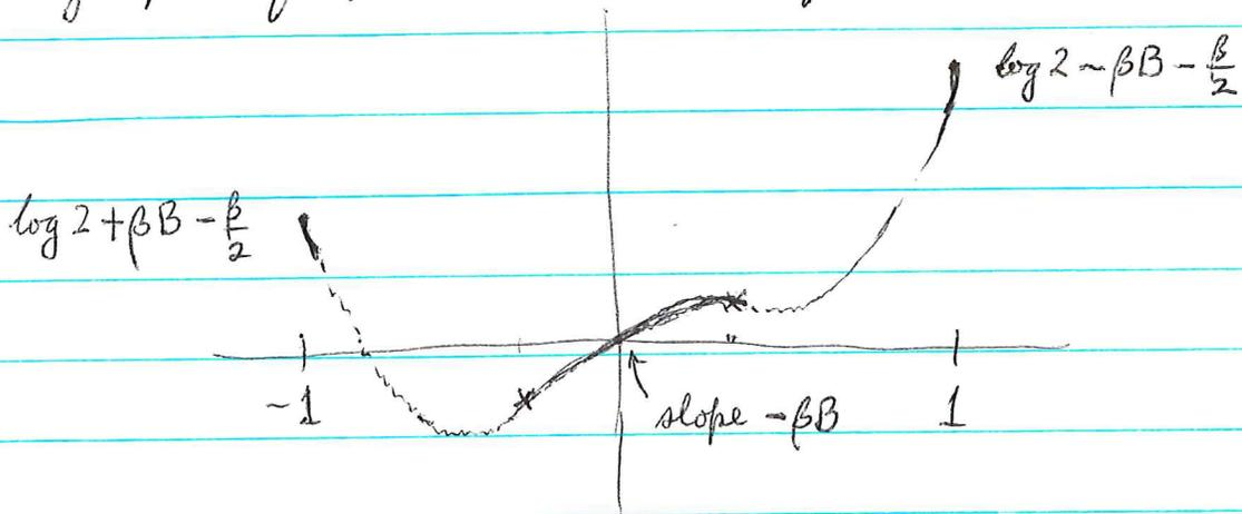
Also  $f''(s) = \frac{1}{1-s^2} - \beta$ . If  $\beta < 1$ , the graph is concave upward and can have only one minimum point necessarily  $< 0$ , (assuming  $B < 0$ ). Otherwise you ~~have~~ have two inflection points and possibly a local minimum for  $s > 0$  as drawn. In any case it's clear that we have a unique minimum point for  $B \neq 0$  ~~no~~ no matter what  $B, \beta$  are. (Notice that even for  $\beta > 1$  the graph is obtained by shearing the case  $B=0$ :
