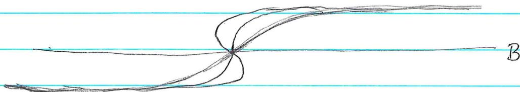
For small  $\bar{s}$ ,  $B \approx \left(\frac{1}{\beta} - gN\right)\bar{s}$  so the curve has slope  $\frac{1}{\frac{1}{\beta} - gN} = \frac{\beta}{1 - \beta gN}$  and the phase transition occurs
