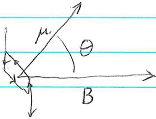
$$\text{Work} = \int_0^\pi \mu B \sin \theta \, d\theta = \left[ -\mu B \cos \theta \right]_0^\pi = 2\mu B$$
