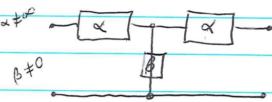
where the boxes denote impedances. We can break  $\beta$  up into two get a 2-port cascades with its reverse.
