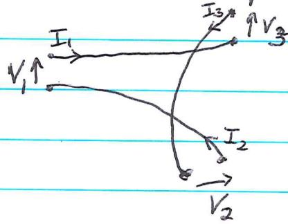
so that  $I_1 = I_2 = I_3$ ,  $V_1 + V_3 + V_2 = 0$ . Then the impedance  $\boxed{\text{ }} \text{ relation}$  is
