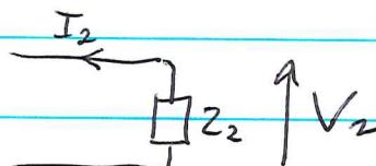
In effect I think of impedance as measuring ratio of voltage to current flowing in:
