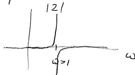
This means the reflection coefficient  $\frac{B}{A}$  is close to  $-1$  for all  $w$  values away from  $\pm 1$ . At these points it sharply shifts to  $+1$ .
