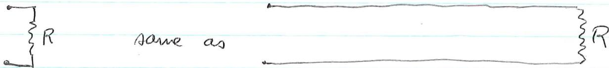
as a length of transmission line of impedance  $R$  terminated by the resistance  $R$ , so there is no reflection. But the transmission line can store energy in its various modes; it behaves like the ether in a cavity. Hence at the temperature  $T$  these modes must be excited like in black body radiation. Thus the resistor  $R$  has to act like a black-body absorbing + emitting energy into the transmission line.
