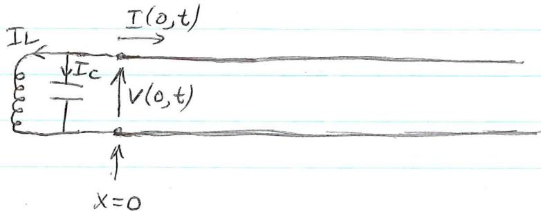
A history of this system is given by functions  $I_L$ ,  $I_C$ , ~~V~~ of  $t$  and function  $I(x,t)$ ,  $V(x,t)$   $x \geq 0$  satisfying the following equations.
